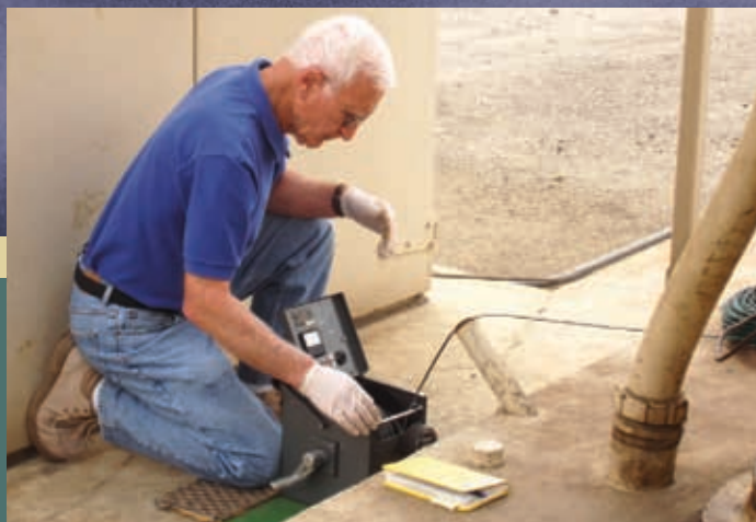
Measuring depth to water in a well.
